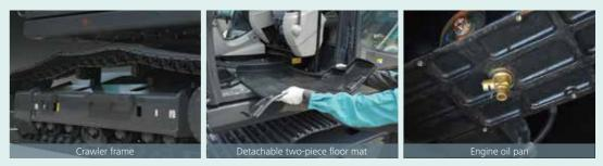
Special crawler frame design is easily cleaned of mud.
