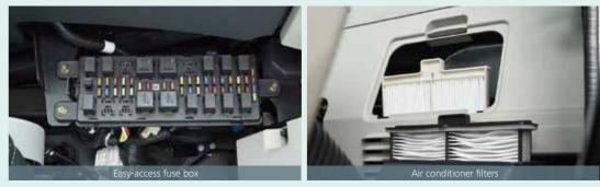
More finely differentiated fuses make it easier to locate malfunctions.
