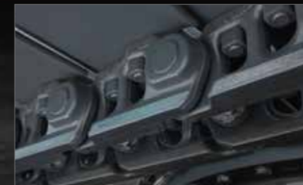
Track Links The size and durability of the track link are increased compared to standard models.
