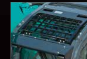
Standard Overhead Top Guard Level II The standard overhead cab guard can be tilted open for easy window cleaning.
