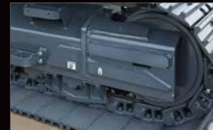
Reinforced Guide Frame ① Reinforced guide frame prevents deformation caused by impact or encroaching of loose stones.
