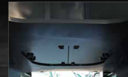
Lower Frame Underside Cover Hydraulic piping and equipment protected against damage from rubble and stony ground.
