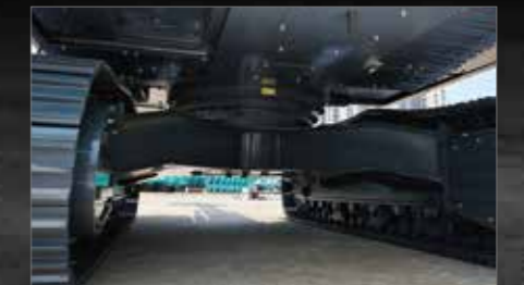
Upper Under Covers Thick covers with increased durability compared to standard models.
