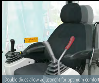
Double slides allow adjustment for optimum comfort
