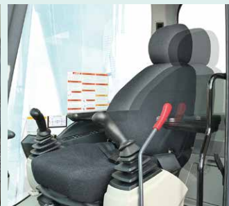
Double slides allow adjustment for optimum comfort
