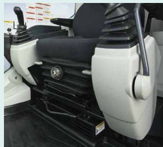
Seat suspension absorbs vibration
