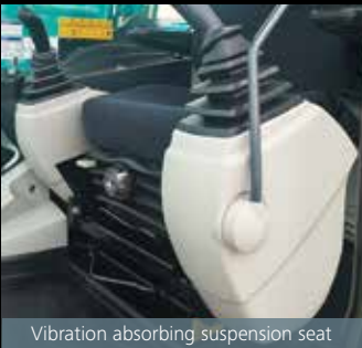
Vibration absorbing suspension seat
