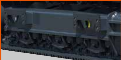
Reinforced track guides Reinforced track guides installed on three places help prevent the crawlers from coming off the rollers.
