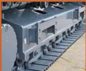
Travel motor protection Large travel motor protectors repel stones and prevent damage to travel motors.
