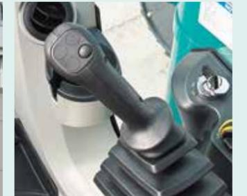
It takes 38%\* less effort to work the operation lever, which reduces fatigue over long working hours or continued operations.
