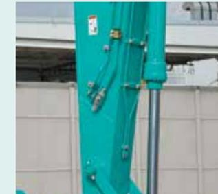
A quick hitch hydraulic line, which speeds up attachment changes, is available as an option.
