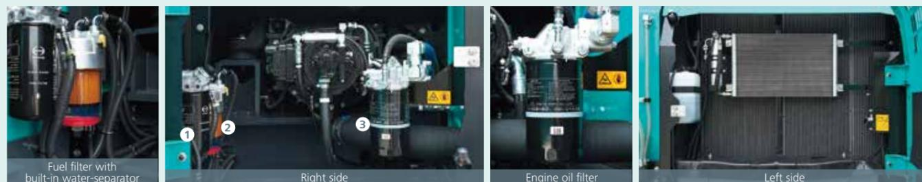
Fuel filter with built-in water-separator
