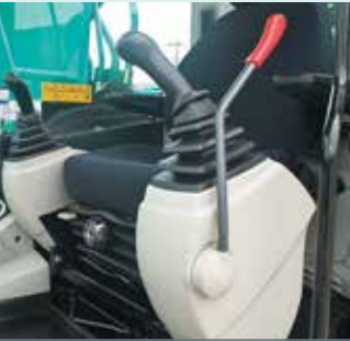
Seat suspension absorbs vibration
