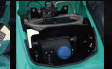
Urea tank Urea filter cap is placed on the step for easy access.
