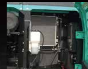
Left side (radiator and cooling system elements) Laid out for easy access to radiator and cooling system.
