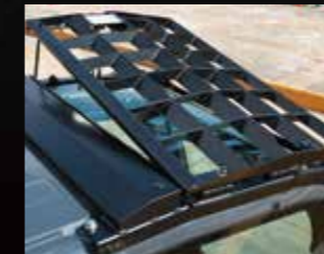
Standard FOPS overhead cab guard The standard FOPS guard can be tilted open for easy window cleaning. Meets standard FOPS, Top Guard Level II requirements. (ISO10262)
