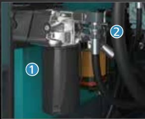
① Fuel Filter ② Pre-Filter with Integrated Water Separator
