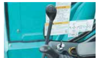
●Travel speed select switch ※The switch is equipped with the dozer lever. (Option)
