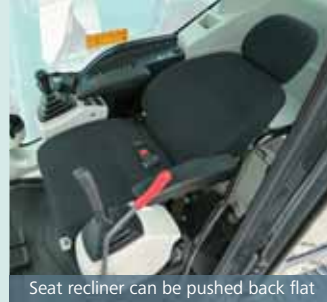
Seat recliner can be pushed back flat
