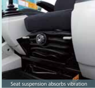
Seat suspension absorbs vibration
