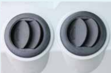
Vents to send cooled air toward the operator if he desires.
