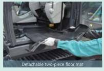
Detachable two-piece floor mat with handles for easy removal. A floor drain is located under floor mat
