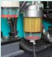
The pre-filter with built-in water-separator has 1.6 times more filter area compared to the previous models and with a new final stage maintenance free fuel filter to maximize filtering performance.
