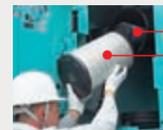
The large-capacity element features a double-filter structure that keeps the engine running clean even in dusty environments.
