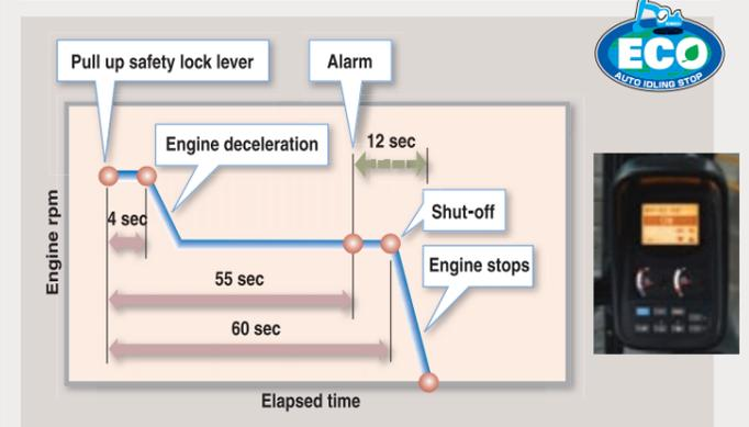
This function saves fuel and cuts emissions by shutting down the engine automatically when the machine is on stand by. It also stops the hourmeter, which helps to retain the machine's asset value.
