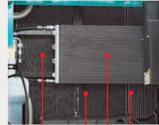
Oil cooler    Radiator    Intercooler
