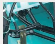
Rigorous inspections for pressure loss are performed on all components of the hydraulic piping, from the first spool of the control valve to connectors. regimen, combined with the use of a new, high-efficiency pump, cuts energy loss to a minimum.
