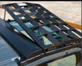
Overhead Top Guard Level II (Optional) The overhead cab guard can be tilted open with gas damper for easy window cleaning. Meets top guard level II requirements. (ISO 10262)
