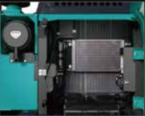
Left Side (Radiator and Cooling System Elements) Laid out for easy access to radiator and cooling system with clean out screen.
