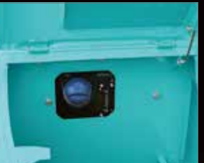
DEF/AdBlue® Tank The DEF/AdBlue® fill is located inside the locking tool box.
