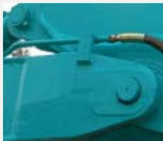
Integrated cast steel boom top
