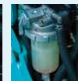
Pre fuel filter with built-in water separator
