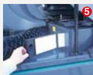
5 Air conditioner filter can be easily removed without tools for cleaning.
