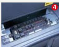
4 Easy-access fuse box. More finely differentiated fuses make it easier to locate malfunctions.
