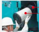
The large-capacity element features a double-filter structure that keeps the engine running clean even in dusty environments.
