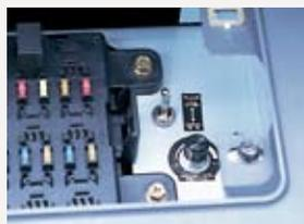
If unexpected trouble is experienced with the ITCS mechatronic control system, the machine can still be operated using the emergency acceleration system. Digging modes are also automatically relayed to an emergency system so that digging can continue temporarily until a service person arrives to repair the primary system.
