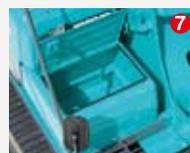
7 Large-capacity tool box can hold up to three pails.
