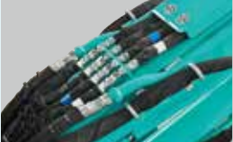
Separation of hoses makes replacement work easier.
