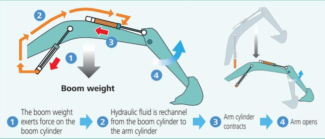
**Hydraulic Circuit Reduces Energy Loss**
