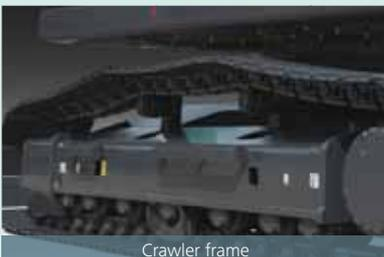
Special crawler frame design for easy mud removal cleaning.
