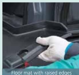
Floor mat's raised edges help keep the cab floor free of mud, simplify cleaning.
