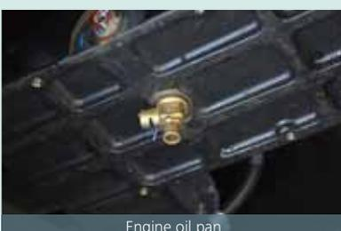
Engine oil pan equipped with drain valve.
