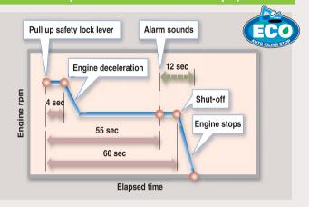
This function saves fuel and cuts emissions by shutting down the engine automatically when the machine is on standby. It also stops the hourmeter, which helps to retain the machine's asset value.
