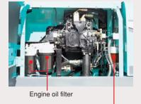
Large fuel filter (with built-in water separator)
