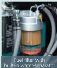
Fuel filter with built-in water-separator
