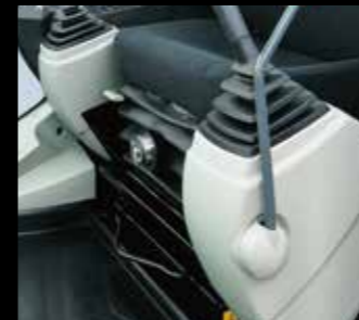
Vibration absorbing suspension seat
