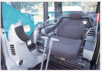
New reclining seat can be lowered well down to the back.
