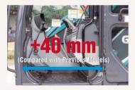
The cab door is 40 mm wider than the previous models, and the control box together with the safety lock lever tilts up by a larger angle, for easy cab entry and exit.
