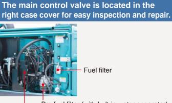
Pre fuel filter (with bult-in water separator) Hydraulic control valve
