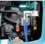
The new engine is a PFRpump fuel injection engine for high reliability. It is equipped with cooled EGR that lowers the temperature of the air intake to reduce its oxygen concentration. It achieves big reductions in particulate matter (PM) and NOx emissions while boosting output.
