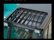
The top guard (FOPS, Top Guard Level II. (Meets ISO10262)) provided as standard. The top-mounted working light ensures
