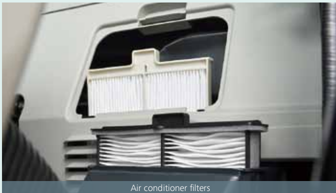
Air conditioner filters
