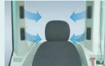
The large air-conditioner has louvers on the back pillars that blow from behind and to the right and left of the operator's seat. They can be adjusted to put a direct flow of cool/warm air on the operator, which means a more comfortable operating environment.
