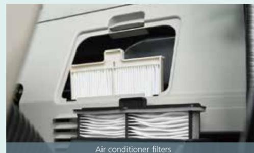
Internal and external air conditioner filters can be easily removed without tools for cleaning.
