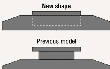
Strength is especially crucial in the carbody. The swing mechanism on the SK850LC is mounted without a column, thereby increasing the carbody's cross-section size for greater strength.
