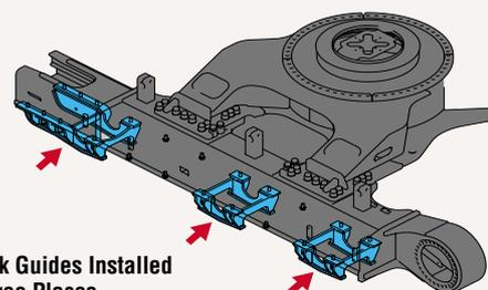
•Track Guides Installed in Three Places
