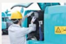
All of the components that require regular maintenance are laid out for easy access. Newly designed, the bonnet opens widely and at a lower level.
