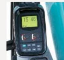
The analog gauge provides information that's easy to read regardless of the operating environment. The information display screen has been enlarged, and a visor is attached to further enhance visibility.
