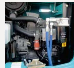
The new engine is a PFR-pump fuel injection engine for high reliability. It is equipped with cooled EGR that lowers the temperature of the air intake to reduce its oxygen concentration. It achieves big reductions in particulate matter (PM) and NOx emissions while boosting output.
