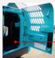
Space is reserved for tools and grease etc., which are necessary for daily maintenance and repair.
