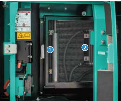
Left side (radiator and cooling system elements)
