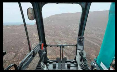
The front window features one large piece of glass without a center pillar on the right side for a wide, unobstructed view.
