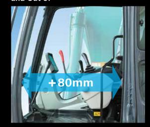
The expanded cab provides plenty of room for a large door, more headroom and smoother entry and exit.
