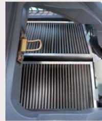
Outside air goes directly from the intake duct through the iNDR filter for dust removal. The filter features a 60-mesh screen, which means it has sixty holes per inch both vertically and horizontally, with a wide front surface area and accordion structure that resists clogging.
