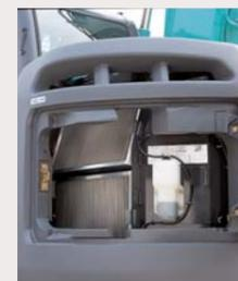
The stainless-steel filter is extremely effective against dust, with a 60-mesh wave-type screen that removes tiny dust particles from the intake air. This not only helps to keep the cooling unit and air cleaner running in top form, but also maintains ideal heat balance.
