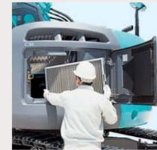
When checking and cleaning the cooling system, one must deal with several different components like the radiator, oil cooler and intercooler, which all must be handled in different ways. But with the iNDR filter, there's just one filter in one place. If it looks dirty during start-up inspection, it can be cleaned easily and quickly.
