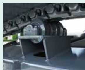
Double-support outer flange upper rollers
