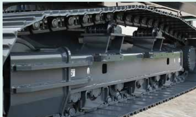
Track guides installed in three places
