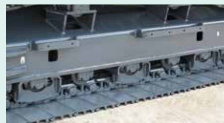
Track guides installed in three places
