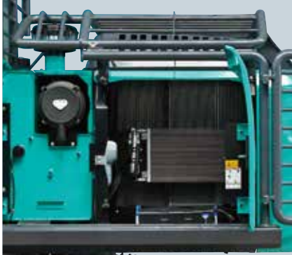
Simple layout for easy access to radiator and cooling system elements
