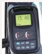
Large analog gauges with large numbers and letters and glare-reducing visors are always easy to read regardless of working conditions.
