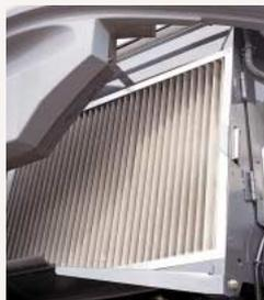
The stainless-steel filter is extremely effective against dust, with a 60-mesh wave-type screen that removes tiny dust particles from the intake air. This not only helps to keep the cooling unit and air cleaner running in top form, but also maintains ideal heat balance.
