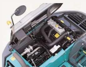
The high-pressure, common-rail fuel-injection engine with the multiple injection system features adjustable control to maximize fuel efficiency and provide powerful low-speed torque. The result is a highly fuel-efficient engine.
