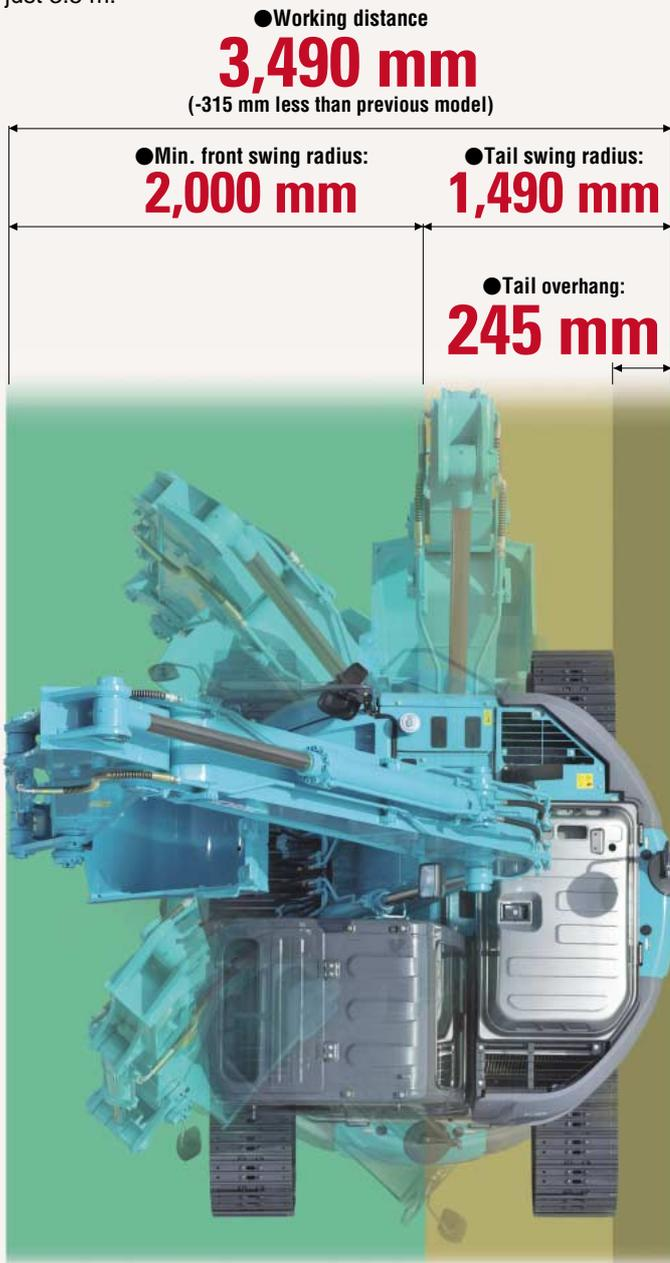
\*"Working distance" equals the sum of the minimum front swing radius and tail swing radius.
