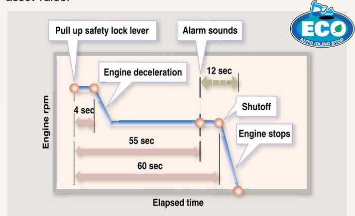
**Automatic Acceleration/Deceleration Function Reduces Engine Speed**
