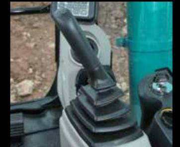
It takes 38% less effort to work the operation lever, which reduces fatigue over long working hours or continued operations.
