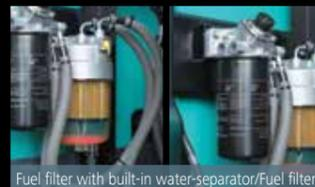
Fuel filter with built-in water-separator/Fuel filter
