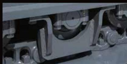
Large, reinforced track guides are installed in three locations.
