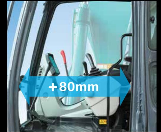
The expanded cab provides plenty of room for a large door, more headroom and smoother entry and exit.
