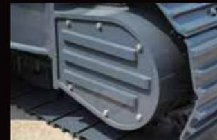
Rear of travel motor cover is reinforced.
