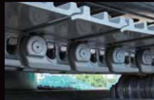
The size and durability of the track link are increased compared to standard models.
