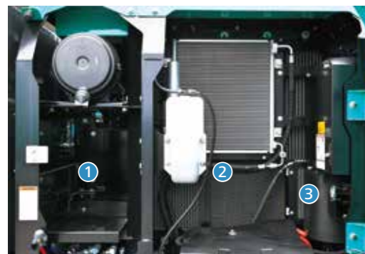
Left side (radiator and tool box space cooling system elements)
