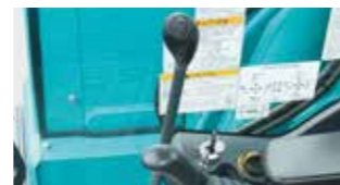
• Travel speed select switch The switch is equipped with the dozer lever.
