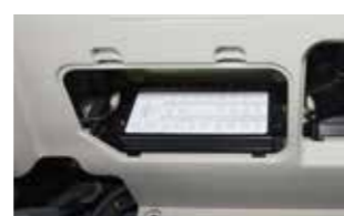
Easy-access fuse box. More finely differentiated fuses make it easier to locate malfunctions.
