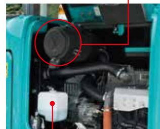
Radiator reservoir tank
