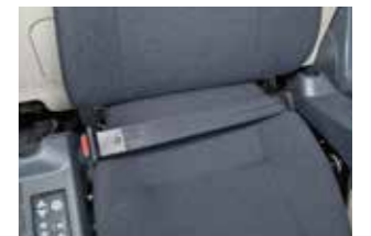
• Retractable seatbelt requires no manual adjustment
