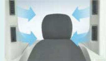
The large air-conditioner has registers on the back pillars that blow from behind and to the right and left of the operator's seat. They can be adjusted to put a direct flow of cool/warm air on the operator, which means a more comfortable operating environment.
