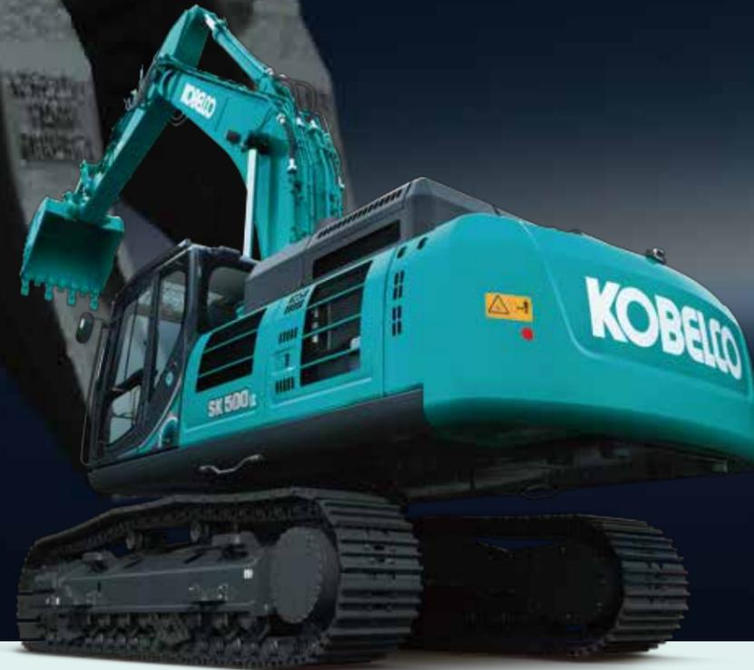
The new arm interflow system more efficiently controls hydraulic fluid flow, and significant reduction of in-line resistance and pressure loss boosts fuel efficiency. The electronic-control common-rail engine features high-pressure fuel injection and multiple injection with improved precision. It is fitted with an EGR cooler which greatly reduce PM and NOx emissions and meets TIERIII Standards.
