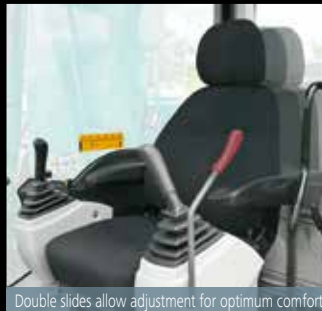
Double slides allow adjustment for optimum comfort
