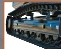
Reinforced track guides installed on three places
