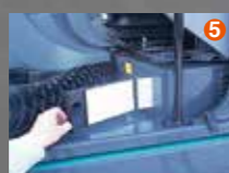
Air conditioner filter can be easily removed.
