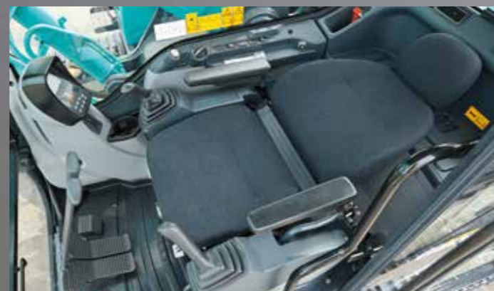
Seat can be reclined to horizontal position
