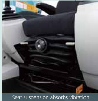
Seat suspension absorbs vibration
