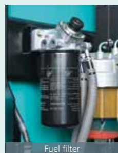
Fuel filter with built-in water-separator
