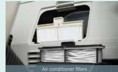
Air conditioner filters
