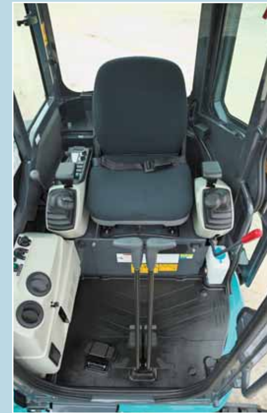
Control levers in photo show HCP lever for optional rotating N&B spec.
