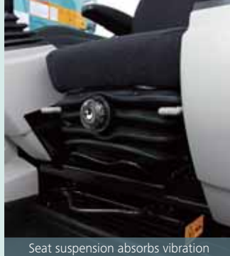
Seat suspension absorbs vibration
