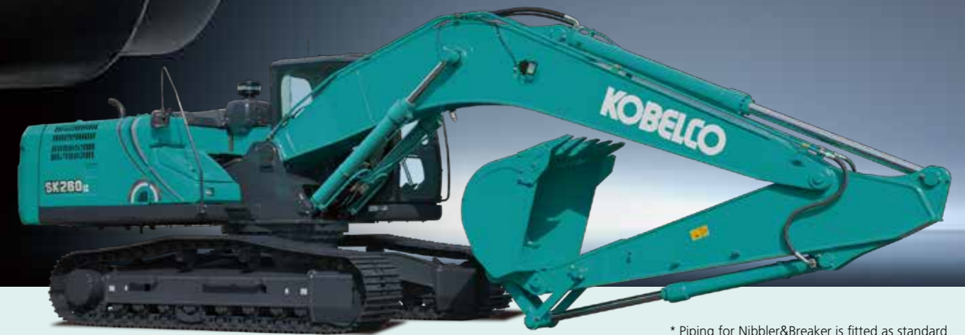
* Piping for Nibbler&Breaker is fitted as standard
